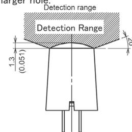
**Recommended Hole Drilling Diameter**
